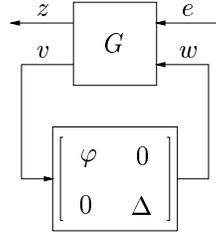
Figure 18: The system in Figure 17 on LFT form.
