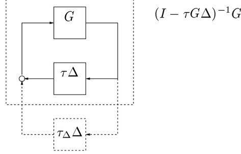
Figure 9: Stability of the feedback interconnection  $(G, \tau\Delta)$  implies stability of the feedback interconnection  $(G, (\tau + \tau_\Delta)\Delta)$  for all  $|\tau_\Delta| \leq \gamma$ , where  $\gamma$  is independent of  $\tau$ . This means that we can insert the dashed branch in the system without losing stability. This allows us to infer stability of  $(G, \Delta)$  through an iterative argument, see Figure 10.
