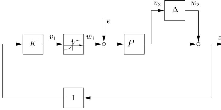
Figure 17: Control system with saturation and uncertainty.
