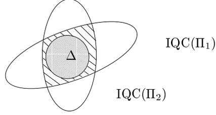
Figure 8: The more IQCs we have the better characterization we get of the uncertainty  $\Delta$ . The grey area represents the set of uncertainties  $\Delta$  and the shaded area represents the complete set of causal bounded operators that satisfy the IQC.
