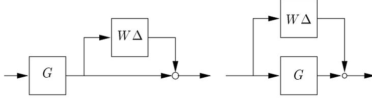
Figure 15: The left block diagram illustrates multiplicative output uncertainty and the right block diagram illustrates additive uncertainty.
