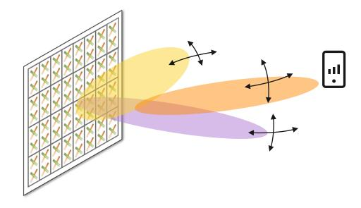
The physical radio channel from base station to user is a MIMO LTI system.
