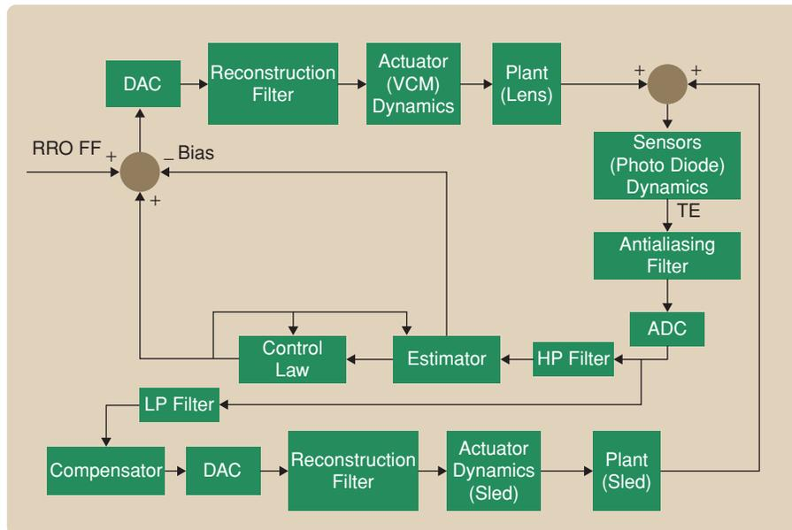
**FIGURE 2** The tracking control loops. The lower (and lower bandwidth) loop commands a motor/gear to position the sled that carries the optical pickup unit (OPU). The higher bandwidth loop drives a voicecoil actuator for fine horizontal positioning of the OPU lens. Repeatable runout (RRO) disturbances are estimated separately and enter as a feedforward term. Not shown is the desired track setpoint.
