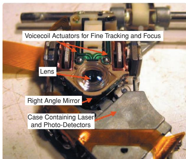
**FIGURE 5** The optical pickup unit. The laser light exits the case at the lower right, is directed upward by the right-angle mirror, and is then focused by the lens. The lens is moved horizontally and vertically by voicecoil actuators.
