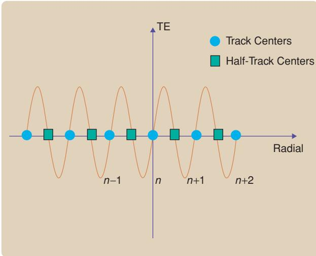
**FIGURE 10** Track error, based on differential push pull, sweeping the lens over tracks. The track error calculated in this method has a sinusoidal appearance. Similar to the track error calculated with the differential push-pull method, zero crossings can be used to count the number of half tracks during a seek, which represents the traveled distance.
