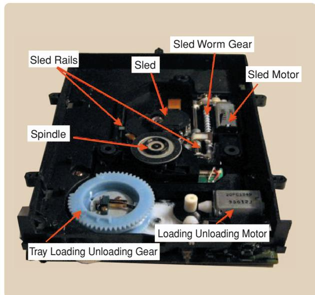
**FIGURE 4** CD drive with tray removed. Under the tray some of the actuators are visible, including the spindle, which spins the disc, the loading and unloading mechanism, and the motor and gear that translate the sled containing the optical pickup unit.
