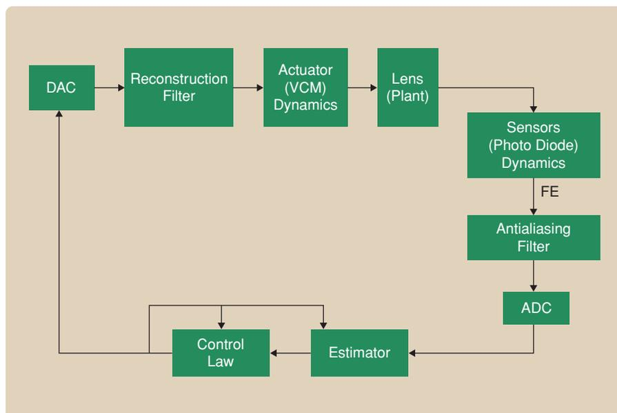
**FIGURE 3** Focus control loop. The bandwidth of focus loop is similar to the bandwidth of the fine tracking loop. An estimator is not needed unless a state-space model similar to the fine-tracking loop is used. An analog circuit calculating the focus error is included in the sensor's dynamics. This circuit can calculate only the distance from the focus point and not the absolute position. Hence the setpoint is eliminated from the diagram.
