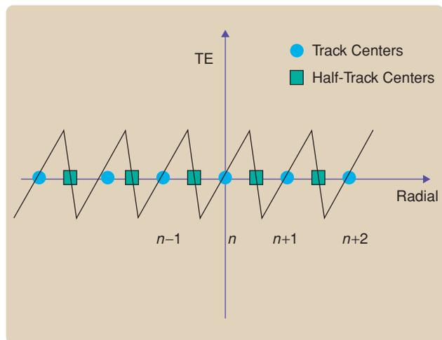
**FIGURE 9** Track error, based on differential phase detect, sweeping the lens over tracks. The track-error signal is capable of showing only the distance from the track center or half-track center. Sweeping the lens over tracks generates a track-error signal that can be used to count the number of half tracks.
