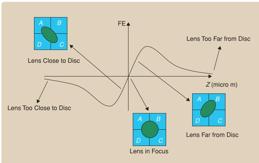
**FIGURE 7** Focus error for a typical arrangement of four detectors. Note the characteristic S-curve generated when the lens is moved up and down. The spot is circular at focus and elliptical when away, while the focus-error signal is small in magnitude when the lens is far away from the disc or close to the disc.
