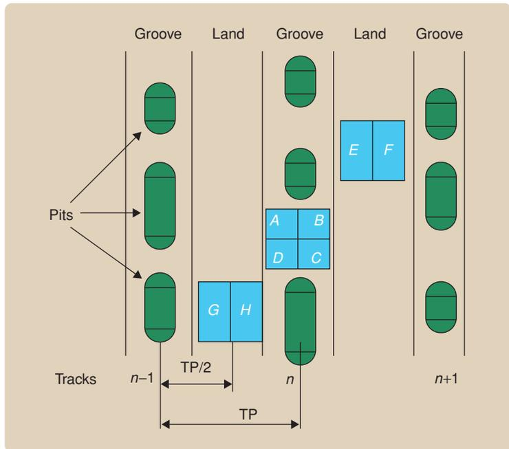
**FIGURE 8** Placement of groove, land, pits, and detectors, including main detectors versus side detectors half a track away. The pits are placed at the center of the groove. The side detectors help measure more accurate track-error signals. Each side detector can be a set of two or four photo diodes. The main detectors are placed on the center of the tracks, while the side detectors are placed at the center of the land, which is also called the half-track. This diagram shows three tracks.
