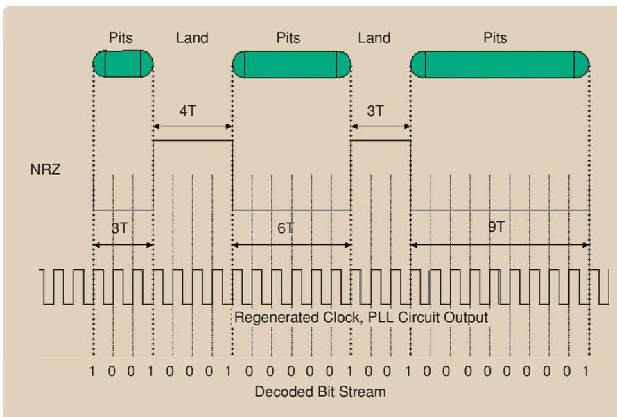
**FIGURE 11** Nonreturn-to-zero signal corresponding to actual bits on the media and regenerated clock from a phase-locked-loop (PLL) circuit. To correctly decode the bit stream, the clock frequency needs to be accurate, which motivates the need for a phase-locked-loop circuit.
