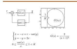
The closed loop system is BIBO stable by the circle criterion.
