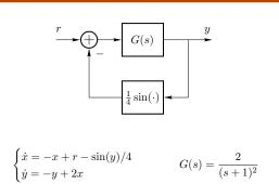
The closed loop system is stable by the small gain theorem.
