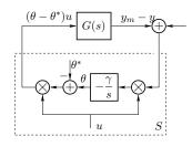
S is passive (Exercise 4.12), so the closed-loop system is BIBO stable if  ${\cal G}(s)$  is strictly passive.
