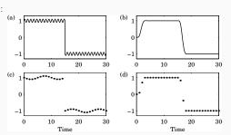
(a), (c):  $f_1=0.9$  Hz,  $f_N=0.5$  Hz  $\Rightarrow f_{alias}=0.1$  Hz
