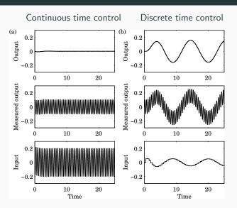
Sampling of high-frequency measurement noise may create new frequencies!
