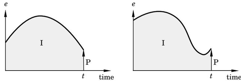
**Figure 2.8** Two control cases where the output from a PI controller are equal at time  $t$ .
