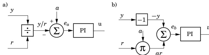
Figure 10.7 Block diagram for two implementations of ratio PI control. The desired ratio of  $y/r$  is  $a$ . The symbol  $\pi$  designates multiplication,  $\div$  designates division.
