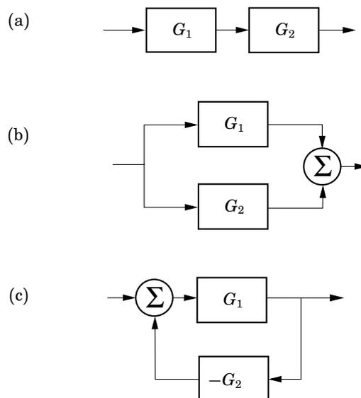
**Figure 4.2** Three basic connections of subsystems: (a) series connection, (b) parallel connection, (c) feedback connection.
