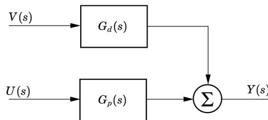
**Figure 8.1** Block diagram of process with input and disturbances.
