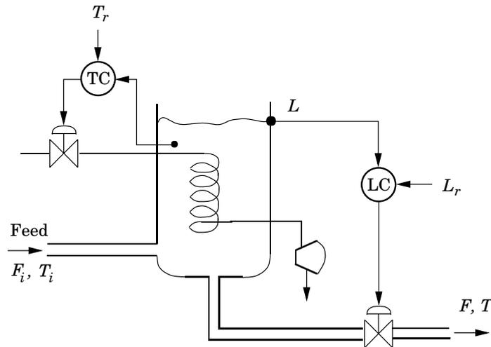
**Figure Y.1** Level and temperature control in a tank.
