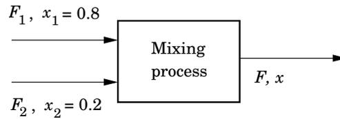
**Figure Y.8** Mixing process, where total flow and mixture should be controlled.
