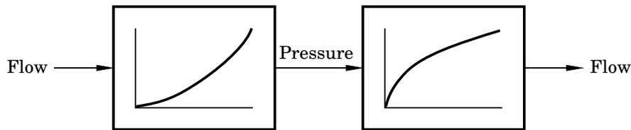
**Figure 5.12** Compensation of the signal from a differential pressure sensor in order to give a flow signal
