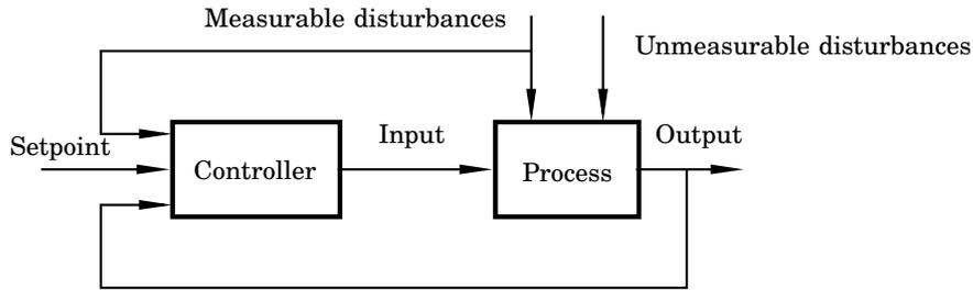
Figure 1.5 A combined feedforward–feedback control system.
