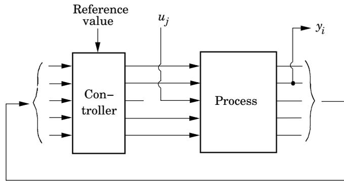
Figure Y.7 A controlled multivariable system.
