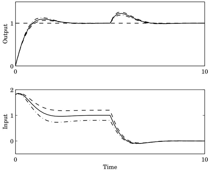
**Figure 6.10** The sensitivity to changes in the flow through the tank, when the system is controlled with a PI-controller with  $K = 1.8$  and  $T_i = 0.45$ . Increase of 20% (dashed), decrease of 20% (dash-dotted), and the nominal case (full). Compare Fig 6.9.
