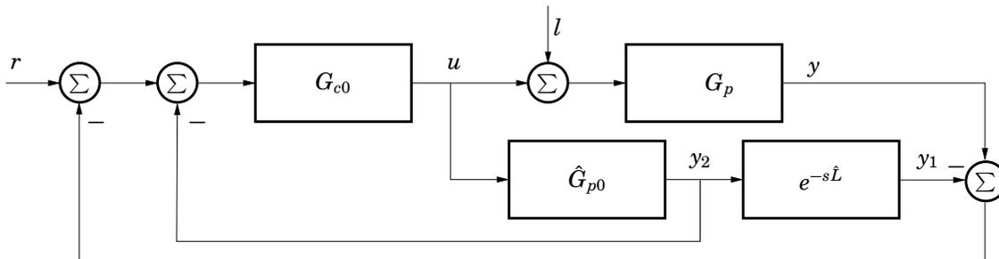
**Figure 10.15** Equivalent structure of the Smith predictor.
