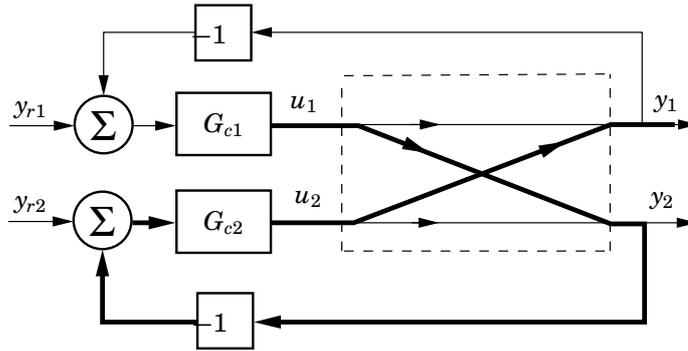
**Figure Y.6** Illustration of the influence of  $u_1$  on  $y_1$  through the second loop.
