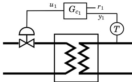
**Figure 10.1** Temperature control of a heat exchanger.
