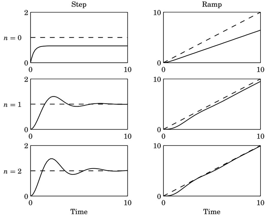
**Figure 7.2** The output and reference values as functions of time for different number of integrators,  $n$ , when the reference signal is a step or a ramp.
