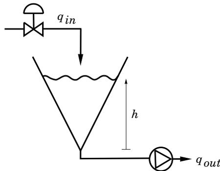
**Figure 6.2** The nonlinear tank in Example 6.2.
