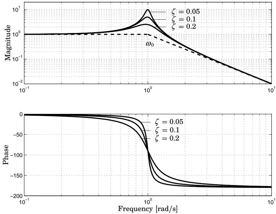
**Figure 8.9** Bode plot of  $G(s) = \omega_0^2 / (s^2 + 2\zeta\omega_0s + \omega_0^2)$ , where  $\omega_0 = 1$  and  $\zeta = 0.05, 0.1, 0.2$ .
