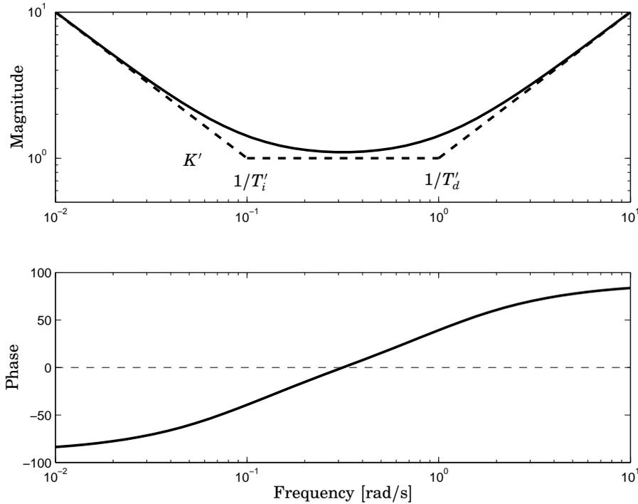
**Figure 9.6** Bode plot of the PID controller with parameters  $K' = 1$ ,  $T_i' = 10$  and  $T_d' = 1$ .
