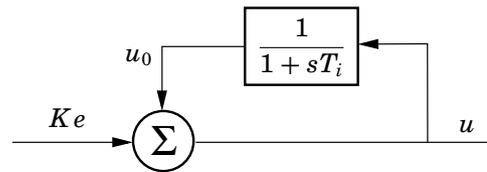
**Figure 9.2** Controller with automatic reset.
