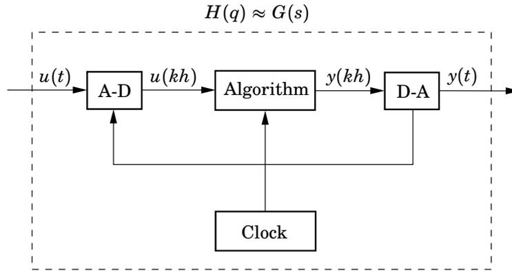
**Figure X.9** Approximating a continuous time transfer function,  $G(s)$ , using a computer.
