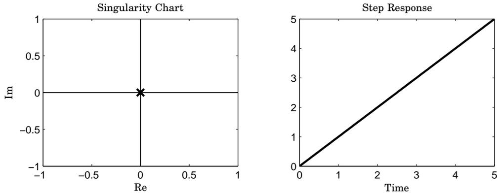
**Figure 5.3** Singularity chart and step response for the process  $G(s) = 1/s$ .
