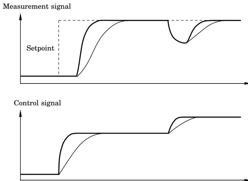
**Figure 10.14** Comparison between the Smith controller (thick lines) and a PI controller (thin lines). The figure shows the control performance when a setpoint change is followed by a load disturbance.
