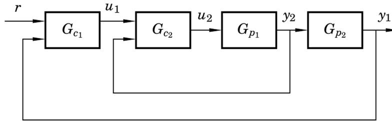
Figure 10.3 The principle of cascade control.
