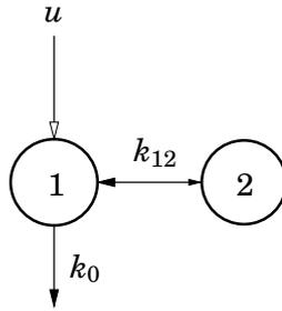
**Figure 3.2** A two-compartment model
