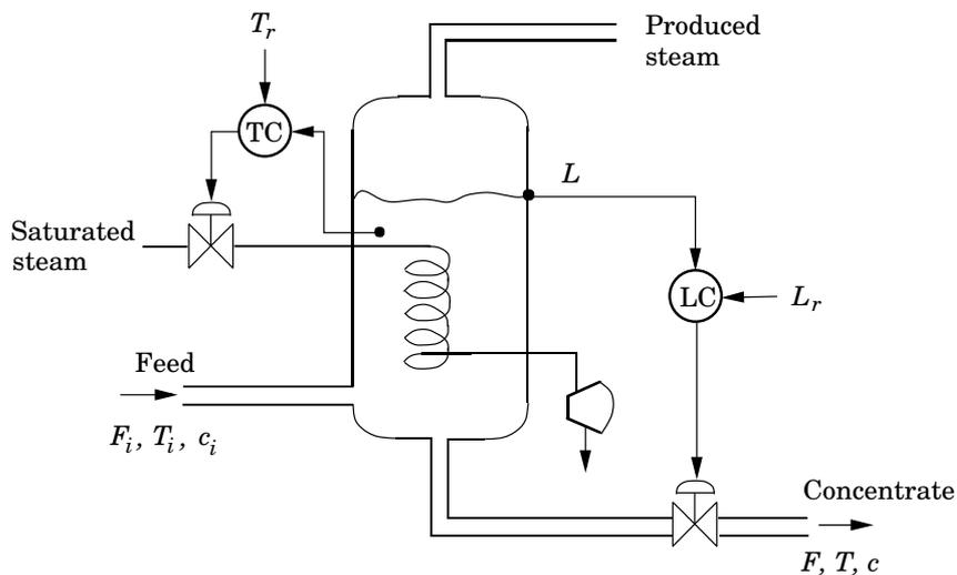
**Figure Y.2** Level and temperature control in an evaporator.
