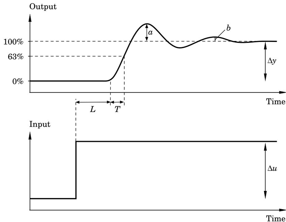
**Figure 2.2** Typical step response with definitions of some process characteristics.
