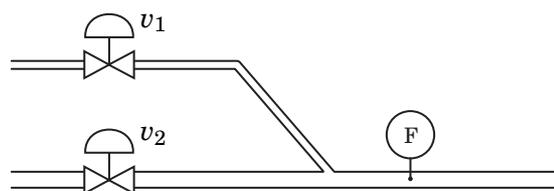
Figure 10.4 Two valves are used to control the flow.
