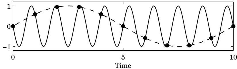
**Figure X.5** Illustration of aliasing. The sinusoidal signals have the frequencies 0.1 and 0.9 Hz respectively. The sampling frequency is 1 Hz.
