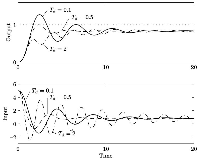
**Figure 9.5** Illustration of the damping properties of derivative action. The process has the transfer function  $G_p(s) = (s + 1)^{-3}$ . The gain is  $K = 5$  and  $T_d$  is varied.
