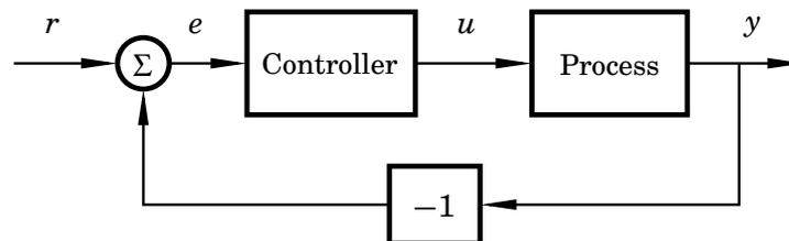
Figure 2.1 A simple feedback loop.
