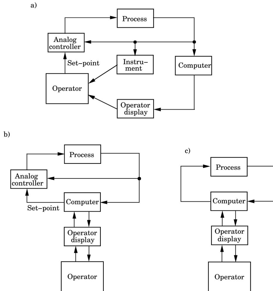
**Figure X.1** Different ways to use computers. a) Operator guide; b) Set-point control; c) Direct Digital Control (DDC).
