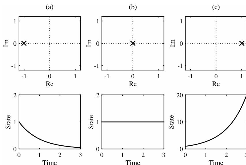
**Figure 3.3** Relationship between eigenvalue location (top) and free system response (bottom) for a first-order system: (a) asymptotic stability, (b) marginal stability, (c) instability. The initial state is  $x(0) = 1$ .
