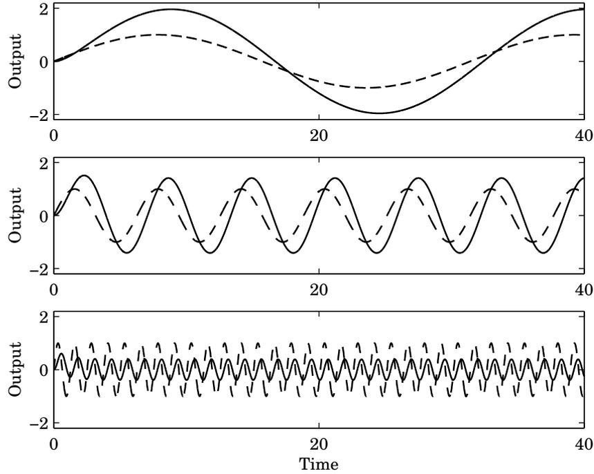
**Figure 8.2** The input (dashed) and output (full) when the signal  $\sin \omega t$  is applied to the system (8.1) with zero initial value, when  $a = 1$ ,  $b = 2$ , and (a)  $\omega = 0.2$ ; (b)  $\omega = 1$ ; (c)  $\omega = 5$ .
