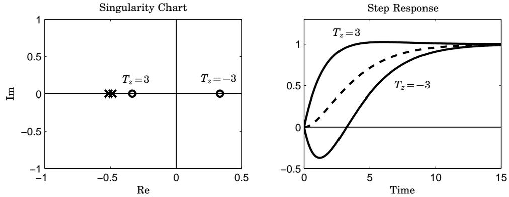
**Figure 5.8** Singularity chart and step response of the process  $G(s) = (1 + sT_z)/(1 + sT)^2$  when  $T_z = 3, -3$ . The dashed step response corresponds to  $G_0(s) = 1/(1 + sT)^2$ , i.e., the process without a zero.
