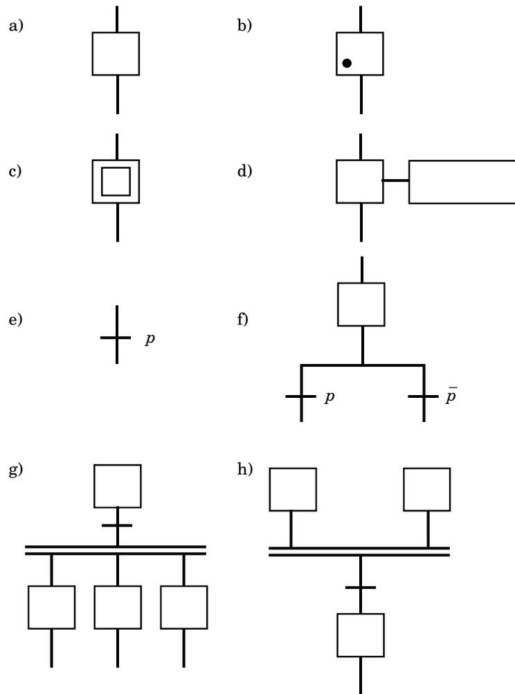
**Figure X.19** GRAFCET symbols. (a) Step (inactive); (b) Step (active); (c) Initial step; (d) Step with action; (e) Transition; (f) Branching with mutually exclusive alternatives; (g) Branching into parallel paths; (h) Synchronization.
