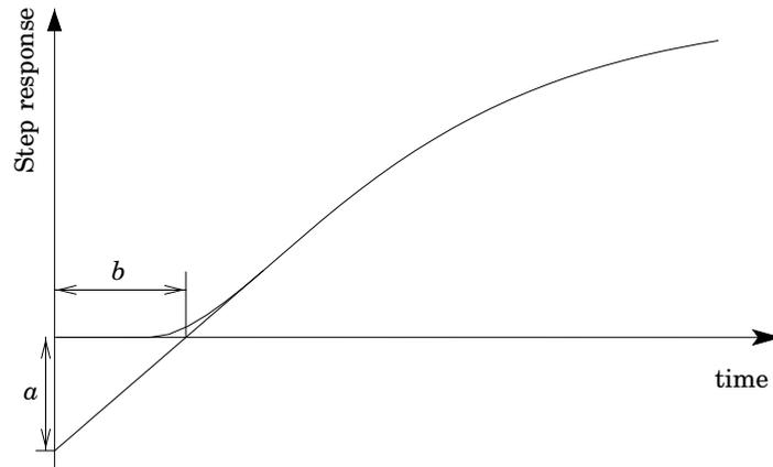
**Figure 9.11** Evaluation of the gain  $a$  and time  $b$  from a process step response.
