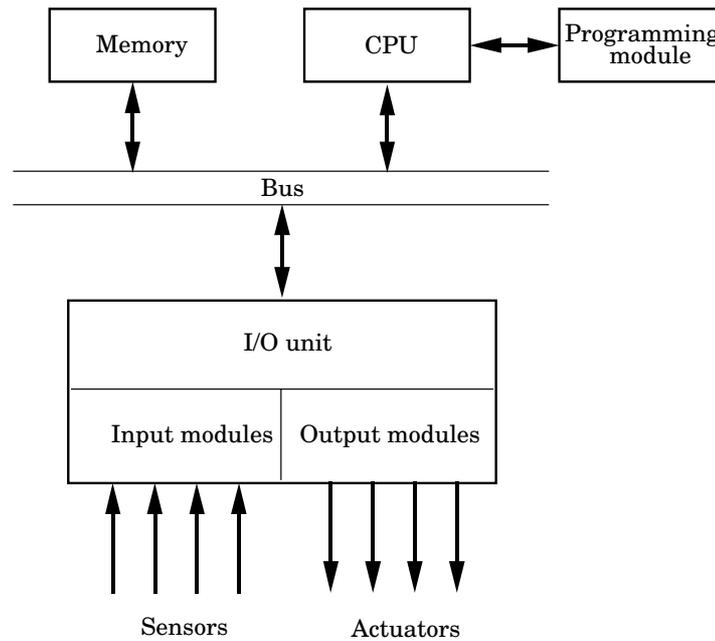
**Figure X.15** Block diagram for a PLC system.
