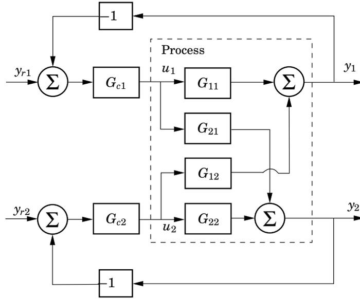
**Figure Y.4** Block diagram of a system with two inputs and outputs. The system is controlled by two simple controllers  $G_{c1}$  and  $G_{c2}$ .
