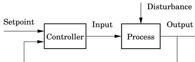
**Figure 1.1** A simple feedback control system.
