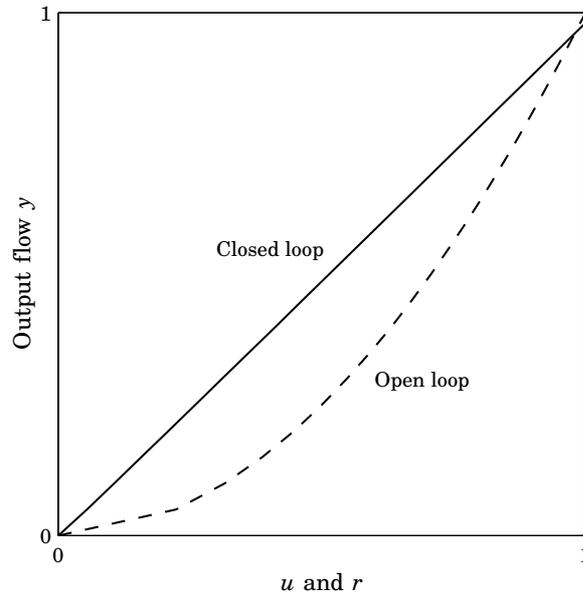
**Figure 7.4** Input-output relations for the open loop system and the closed loop system when  $K = 50$ . Notice that the input for the open loop system is  $r$  for the closed loop system.
