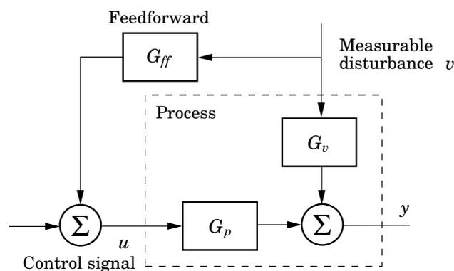
Figure 10.9 System with measurable disturbance.
