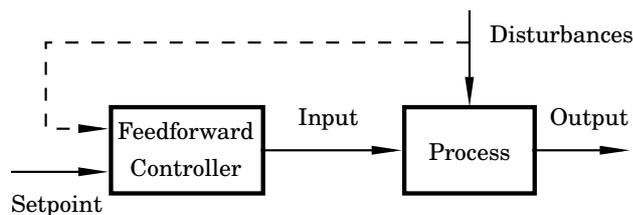
**Figure 1.4** A feedforward control system.
