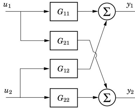
**Figure Y.3** Coupled system with two inputs and two outputs.
