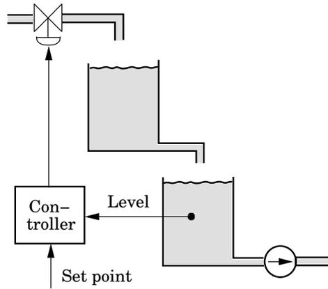
Figure X.10 Level control of a two-tank system.
