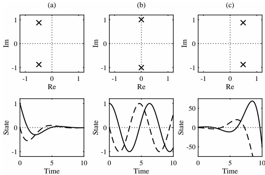
**Figure 3.4** Relationship between eigenvalue locations (top) and free system response (bottom) for a second-order system: (a) asymptotic stability, (b) marginal stability, (c) instability. The initial state is  $x(0) = [1 \ 0]^T$ .
