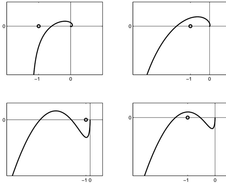
**Figure 8.12** Nyquist curves for four different loop transfer functions. According to the Nyquist criterion the two leftmost systems are stable, whereas the two systems to the right are unstable.
