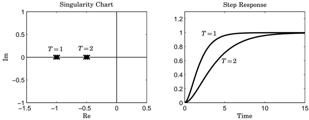
**Figure 5.5** Singularity chart and step response of the process  $G(s) = 1/(1 + sT)^2$  when  $T = 1, 2$ .
