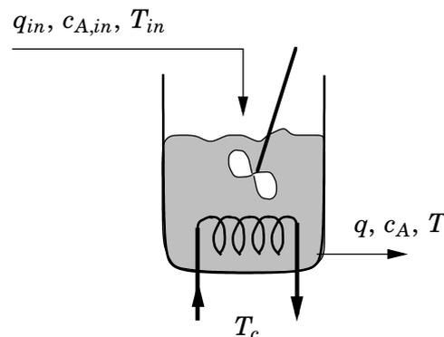
**Figure 3.1** Continuous stirred tank reactor with cooling coil
