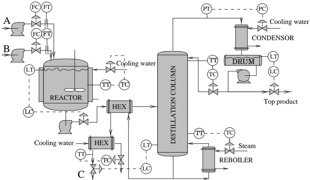
**Figure 1.9** Process and instrumentation (P/I) diagram for the process in Figure 1.8. Signal connections are indicated with dashed lines.
