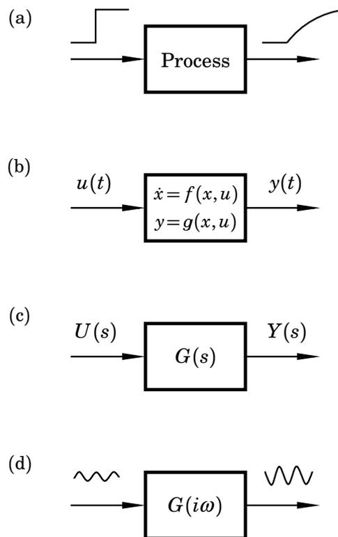
**Figure 1.10** Illustration of some different dynamical process models that will be used in the course: (a) experimental step-response model, (b) nonlinear state-space model, (c) linear input-output model in the Laplace domain, (d) frequency-response model.
