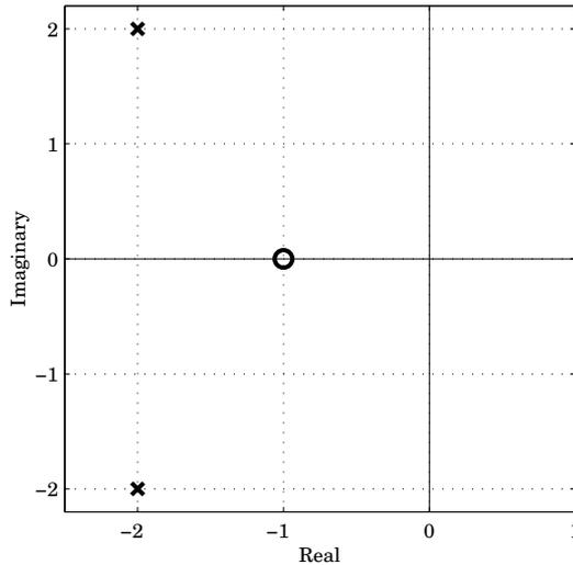
**Figure 4.1** Singularity diagram for the system  $G(s) = k(s + 1)/(s^2 + 4s + 8)$ .
