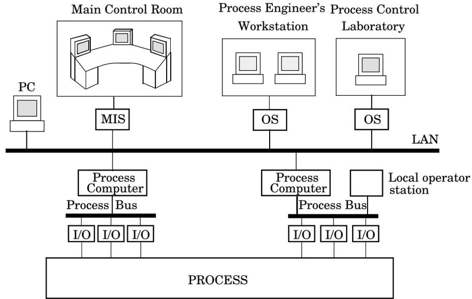
Figure X.3 Architecture of a distributed control system.
