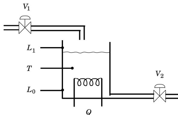
**Figure X.18** Process for batch water heating.
