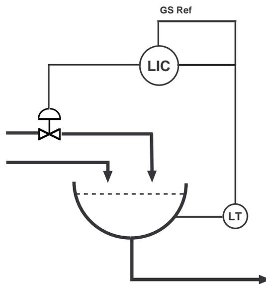
**Figure 5.16** Gain scheduling in the level control of a nonlinear tank
