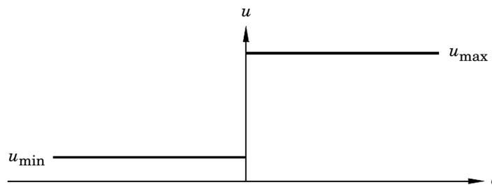
**Figure 2.6** The control signal of the On/Off controller.
