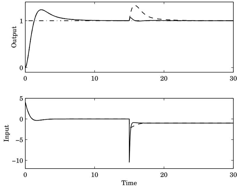
**Figure 10.12** Feedforward and feedback control of the process in Figure 10.10 using (10.1) with  $T_{ff} = 0.1$  and  $\text{bias} = -0.05$ . The feedback controller is a PID controller with  $K_c = 4$ ,  $T_i = 3$ , and  $T_d = 0.5$ . (a) Output with (full) and without (dashed) feedforward; (b) Input with (full) and without (dashed) feedforward. The reference signal is a unit step at  $t = 0$  and the load disturbance is a unit step at  $t = 15$ .
