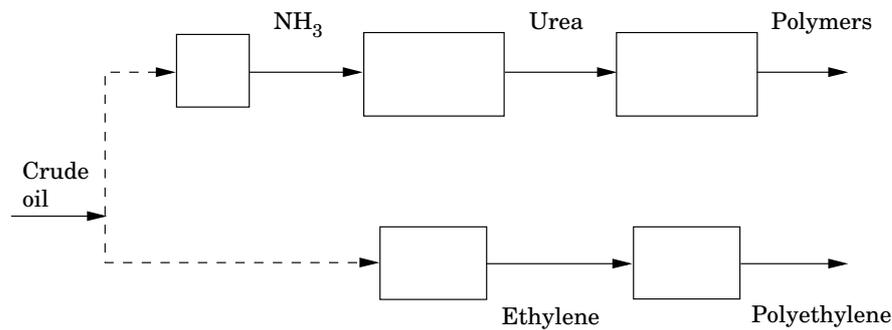
**Figure 1.7** Schematic layout of a more complex plant site.
