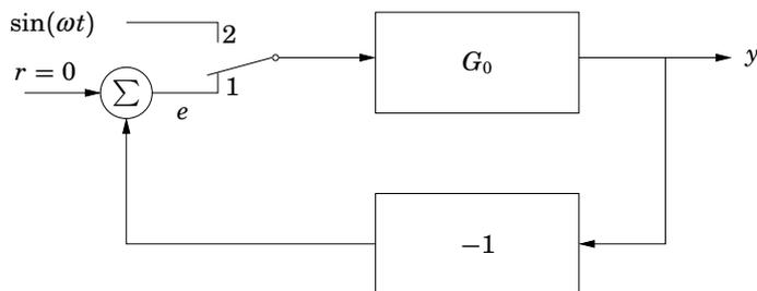
Figure 8.11 The simple feedback loop, being analyzed by means of the Nyquist criterion.
