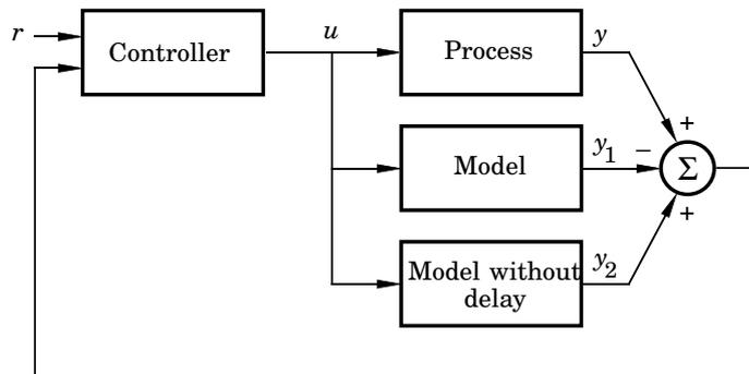
**Figure 10.13** The principle of the Smith predictor.
