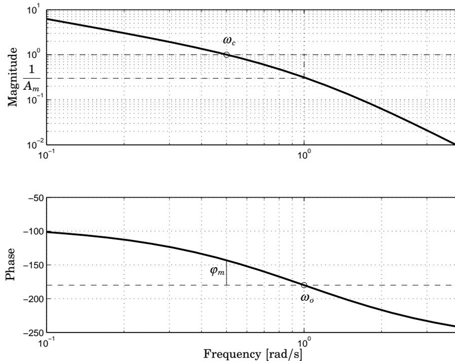
**Figure 8.14** Phase margin  $\varphi_m$  and gain margin  $A_m$  in the Bode plot.
