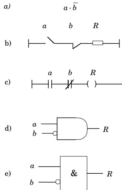
**Figure X.14** Different ways to represent the logical expression  $a \cdot \bar{b}$ : (a) Boolean algebra; (b) Relay symbols; (c) Ladder symbols; (d) Logical circuit symbols (American standard); (e) Logical circuit symbols (Swedish standard).
