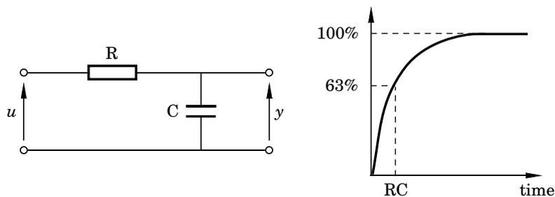
**Figure 2.5** A simple RC circuit and its step response.
