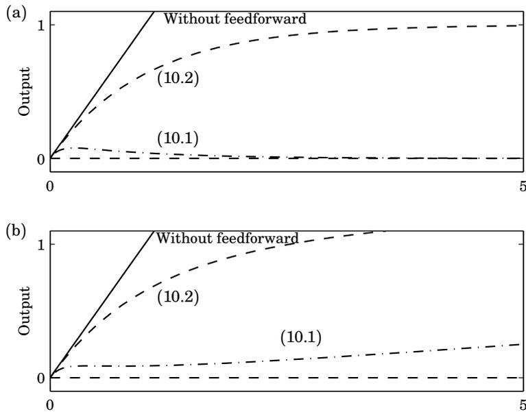
**Figure 10.11** Feedforward control of the process in Figure 10.10 using (10.1) and (10.2) with  $T_{ff} = 0.1$ , when the disturbance is a unit step. The response without feedforward, i.e. the open loop response, is also shown. (a) No measurement bias; (b) Measurement bias 0.05.
