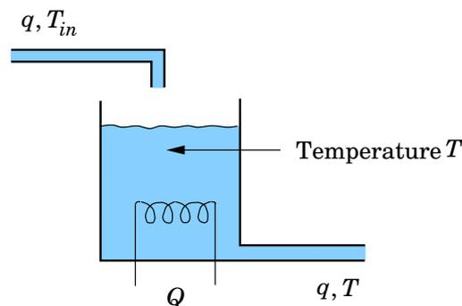
Figure 6.3 Stirred tank process.
