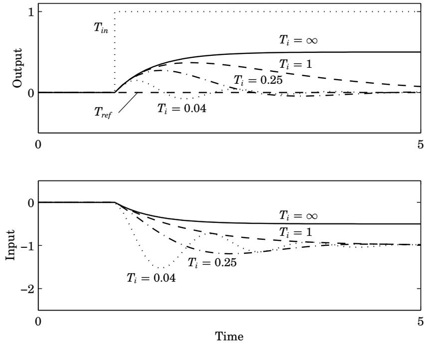
**Figure 6.8** Simulation of the stirred tank under PI control with  $K = 1$  and  $T_i = \infty, 1, 0.25,$  and  $0.04$ . The desired reference value is  $T_{ref} = 0$  and the disturbance is a unit step at  $t = 1$ .
