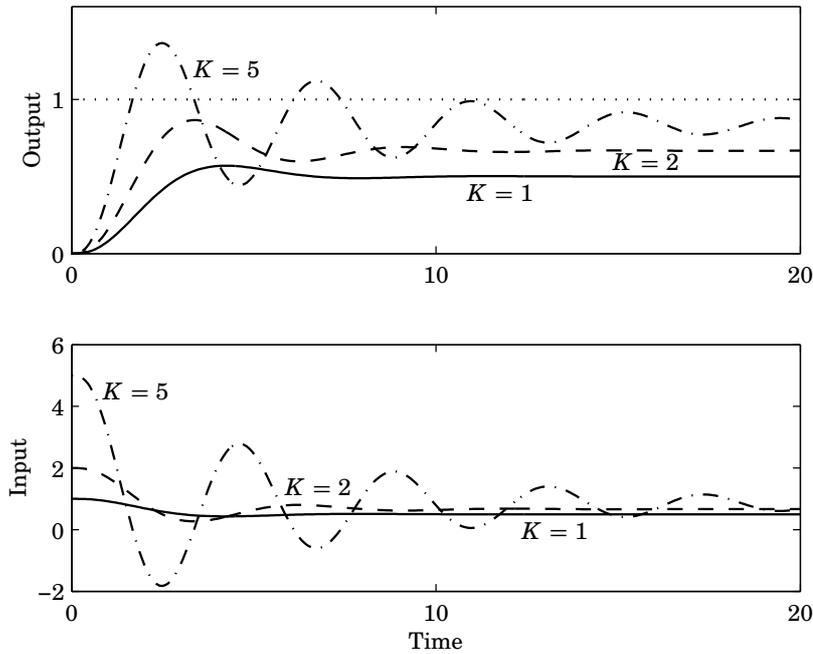
**Figure 9.1** Illustration of proportional control. The process has the transfer function  $G_p(s) = (s + 1)^{-3}$ .
