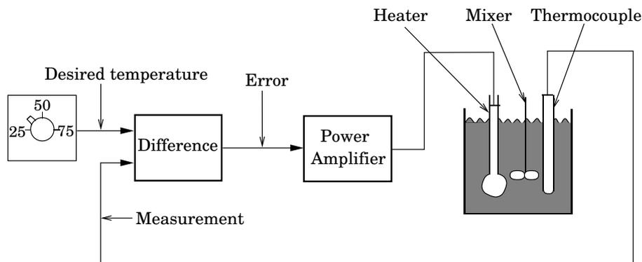
Figure 1.2 A simplified diagram of a thermostat for heating of water.
