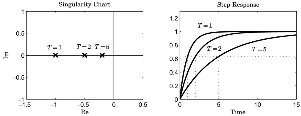
**Figure 5.4** Singularity chart and step response for the process  $G(s) = 1/(1 + sT)$  when  $T = 1, 2, 5$ .
