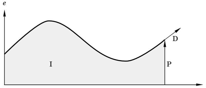
**Figure 2.9** Illustration of PID control. The integral part is proportional to the surface under the control error curve, the proportional part is proportional to the current control error and the derivative part is proportional to the change rate of the control error.
