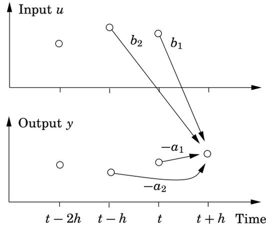
**Figure X.8** Illustration of the difference equation  $y(t) + a_1y(t-h) + a_2y(t-2h) = b_1u(t-h) + b_2u(t-2h)$ .
