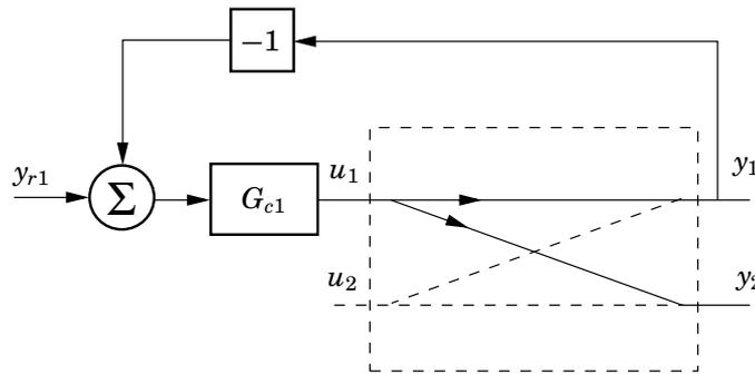
**Figure Y.5** The system in Figure Y.4 when only the first loop is closed.
