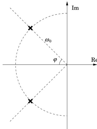
**Figure 5.6** Interpretation of the parameters in the characteristic polynomial  $s^2 + 2\zeta\omega_0s + \omega_0^2$ . The distance between the poles and the origin is the undamped frequency  $\omega_0$ , whereas  $\zeta = \cos \varphi$  is the relative damping of the system.
