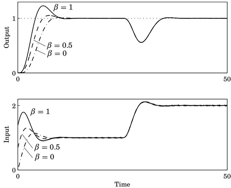
**Figure 9.7** Response of system to setpoint changes and load disturbances for controller with different values of parameter  $\beta$ .
