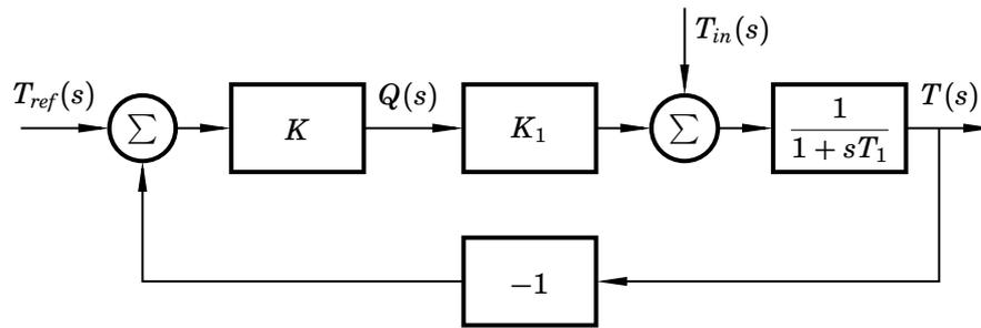
**Figure 6.5** Proportional control of the stirred tank process.
