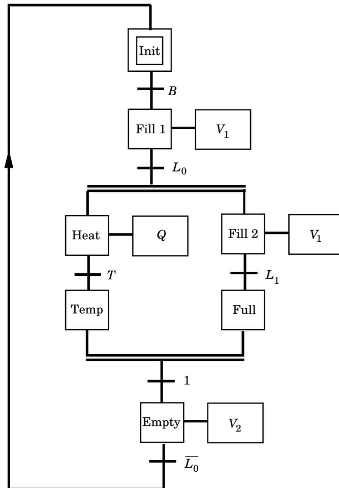
**Figure X.20** GRAFCET for the process and sequences in Example X.9.
