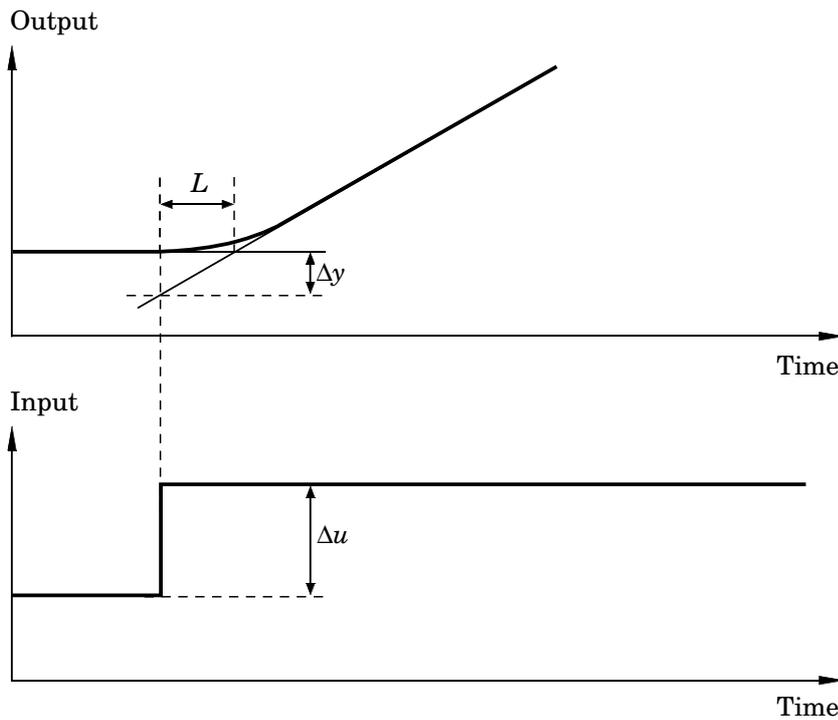
Figure 2.3 Step response for an integrating process.
