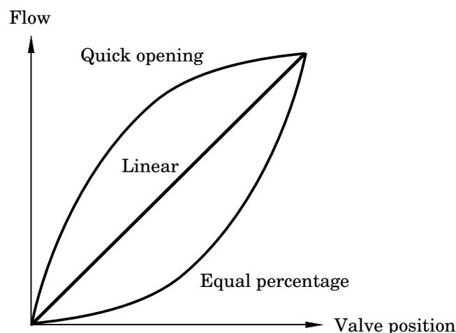
**Figure 5.9** Some different types of valve characteristics
