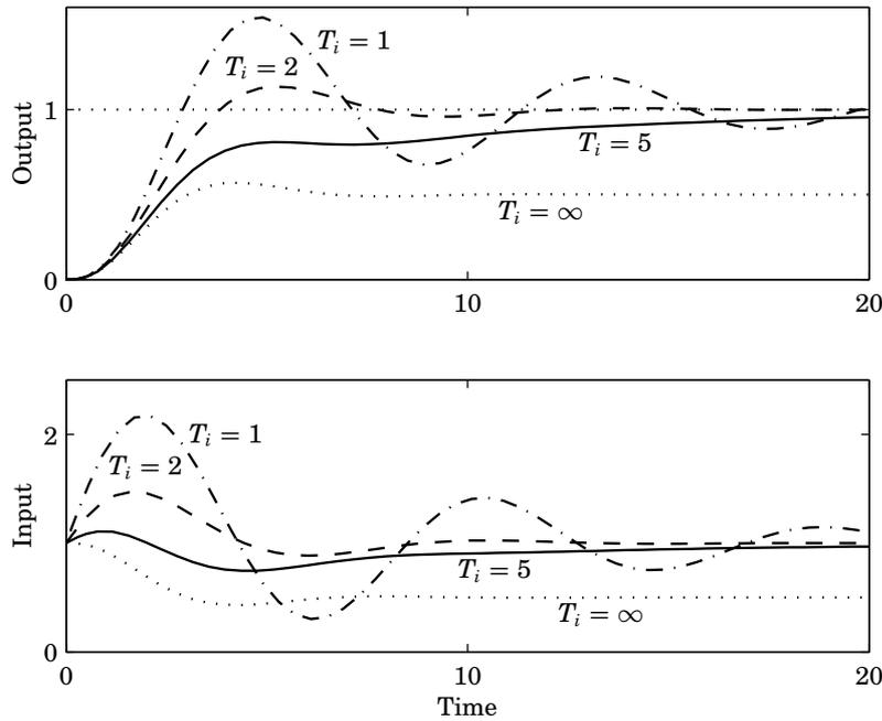
**Figure 9.3** Illustration of PI control. The process has the transfer function  $G_p(s) = (s + 1)^{-3}$ . The controller has the gain  $K = 1$ .
