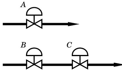
**Figure 5.10** Two cases which will result in different valve characteristics
