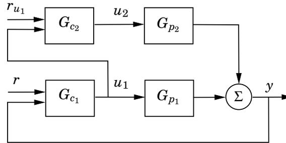
Figure 10.6 Block diagram of a system with mid-range control.
