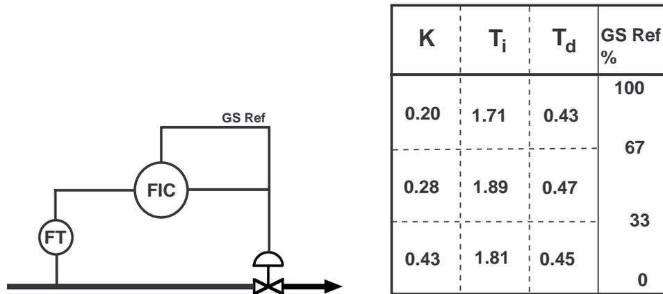
**Figure 5.15** Gain scheduling to compensate for a nonlinear valve
