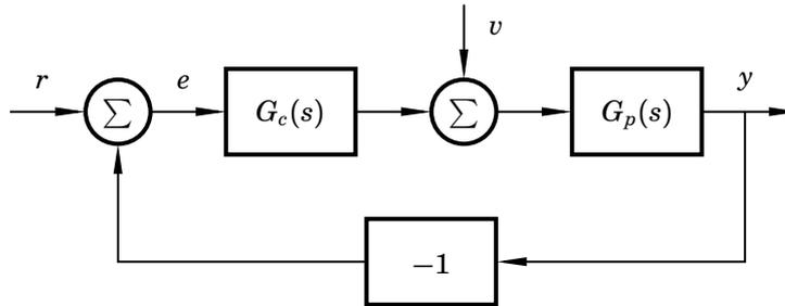
**Figure 7.1** Simple feedback control system with reference signal  $r$  and disturbance signal  $v$ .
