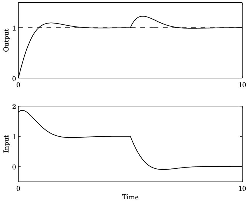
**Figure 6.9** Reference and load disturbance for the temperature control system using a PI-controller  $K = 1.8$  and  $T_i = 0.45$ . The liquid temperature and the control signal are shown.
