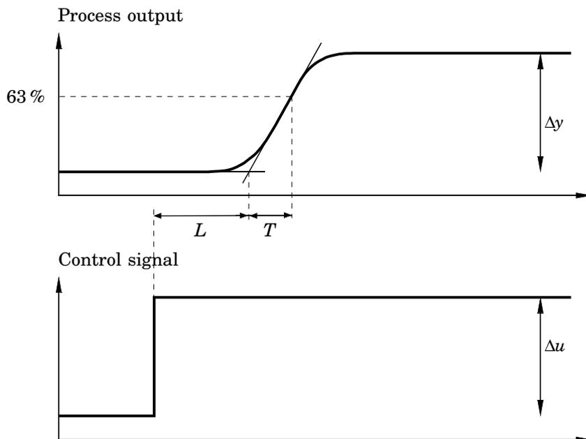
**Figure 9.12** Determination of  $K_p$ ,  $L$ , and  $T$  from a step response experiment.
