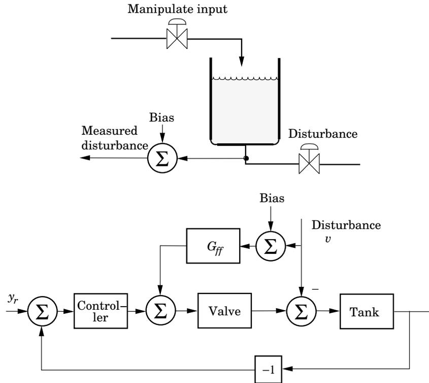
**Figure 10.10** Tank system with measurable disturbance.
