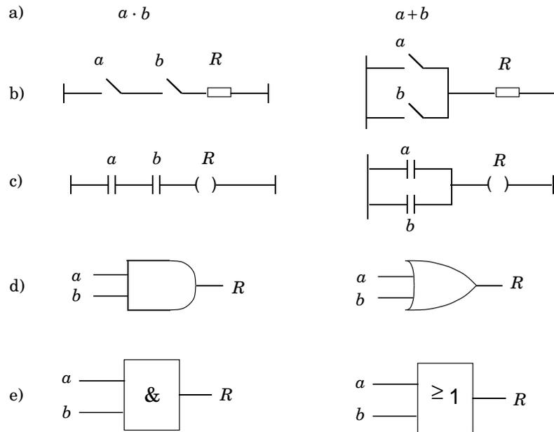
**Figure X.13** Different ways to represent the logical expressions  $a \cdot b$  and  $a + b$ : (a) Boolean algebra; (b) Relay symbols; (c) Ladder symbols; (d) Logical circuit symbols (American standard); (e) Logical circuit symbols (Swedish standard).
