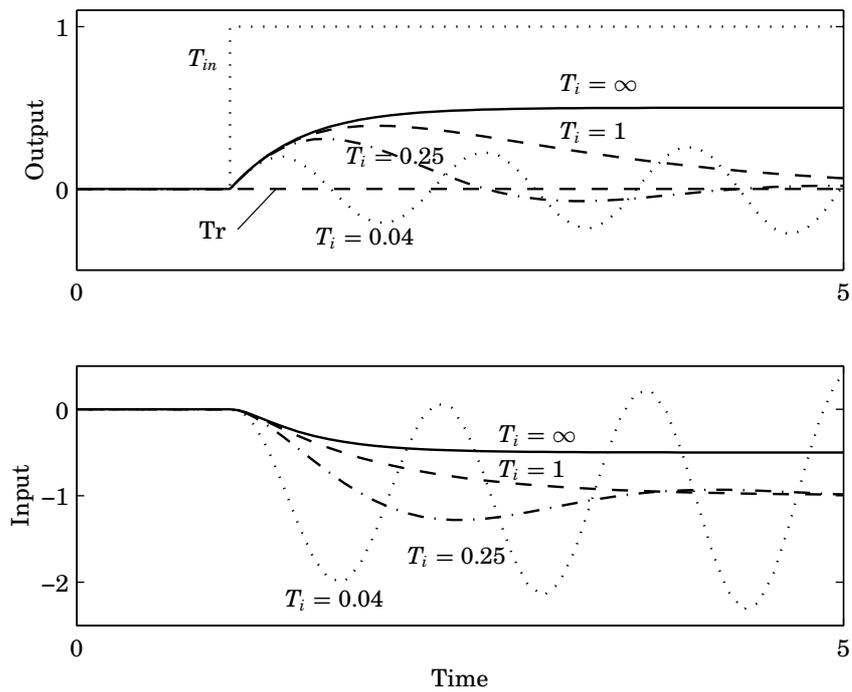
**Figure 6.11** Temperature control using PI-controller and sensor dynamics. The liquid temperature and the control signal are shown when  $T_{in}$  is a unit step,  $T_s = 0.1$ ,  $K = 1$  and  $T_i = \infty$ , 1, 0.25, and 0.04. Compare Figure 6.8
