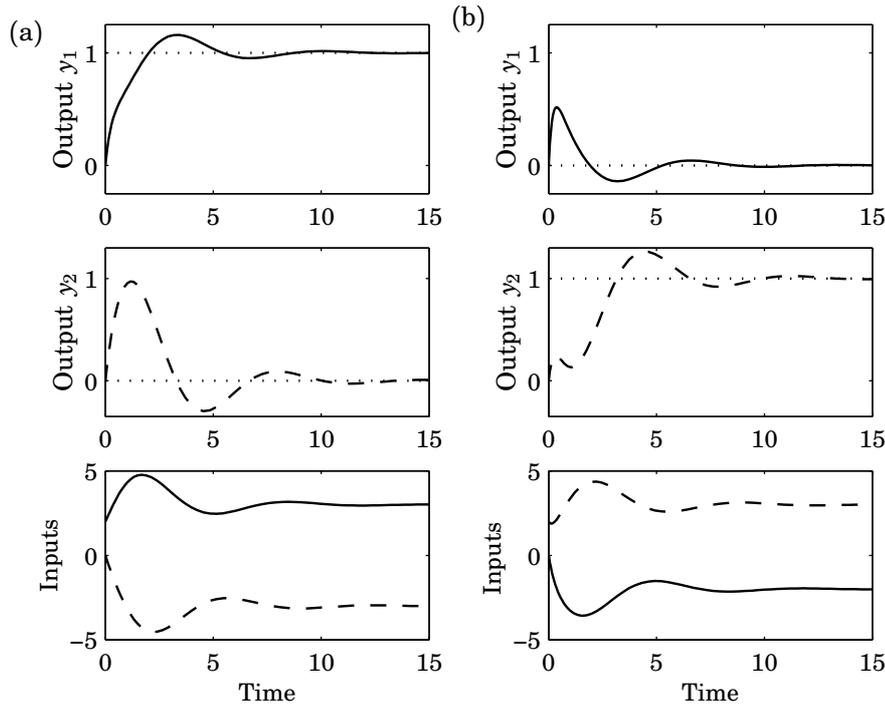
**Figure Y.10** The process in Example Y.8 controlled by two PI controllers. (a)  $y_1$ ,  $y_2$  and the control signals  $u_1$  and  $u_2$ , when the reference value of  $y_1$  is changed. (b) Same as (a) when the reference value of  $y_2$  is changed.
