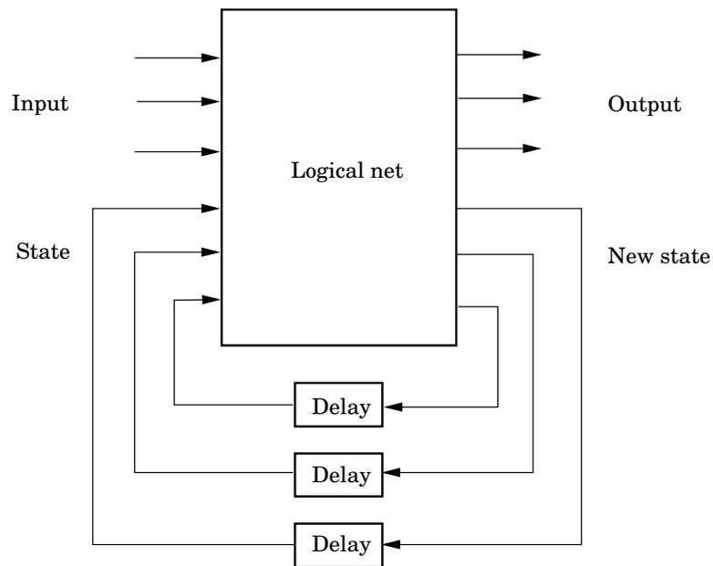
**Figure X.17** Synchronous sequential net as combination of logical net and delay or memory elements.
