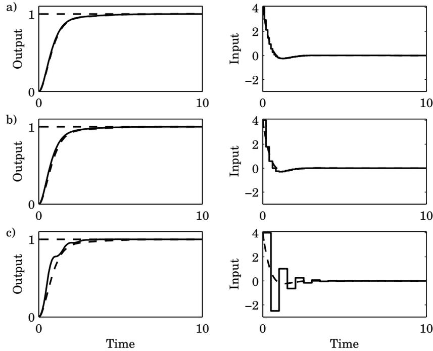
**Figure X.11** Process output and input when the process (X.6) is controlled by (X.7) and the sampled-data controller (X.8) when a)  $h = 0.1$ ; b)  $h = 0.2$ ; c)  $h = 0.5$ . The dashed signals are the output and input when the continuous time controller is used.
