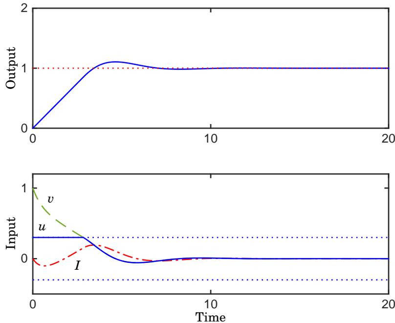
**Figure 9.10** Illustration of controller with anti-windup using tracking. Compare with Figure 9.8.
