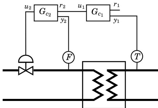
**Figure 10.2** Cascade control of a heat exchanger.
