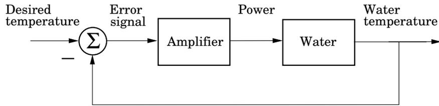
**Figure 1.3** Block diagram of the thermostat in Figure 1.2.
