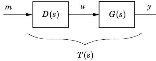
**Figure Y.9** A system with decoupling matrix  $D$ .
