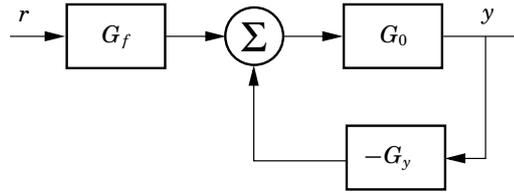
Figure 7.5 Closed-loop system.
