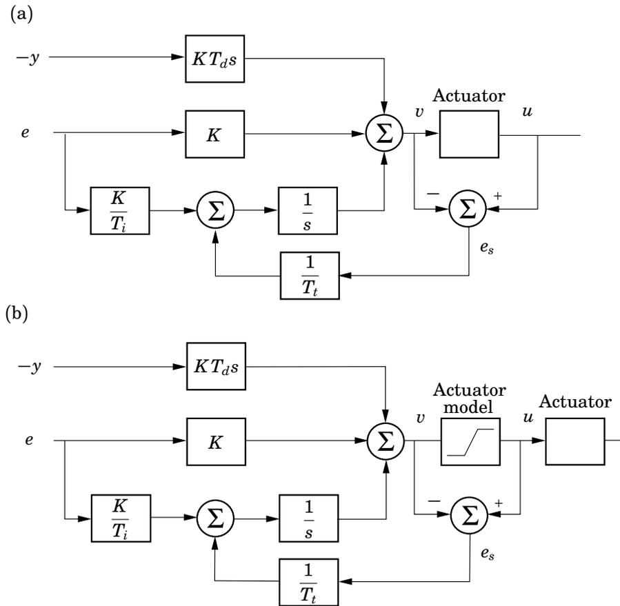
**Figure 9.9** Controller with anti-windup. A system where the actuator output is measured is shown in (a) and a system where the actuator output is estimated from a mathematical model is shown in (b).
