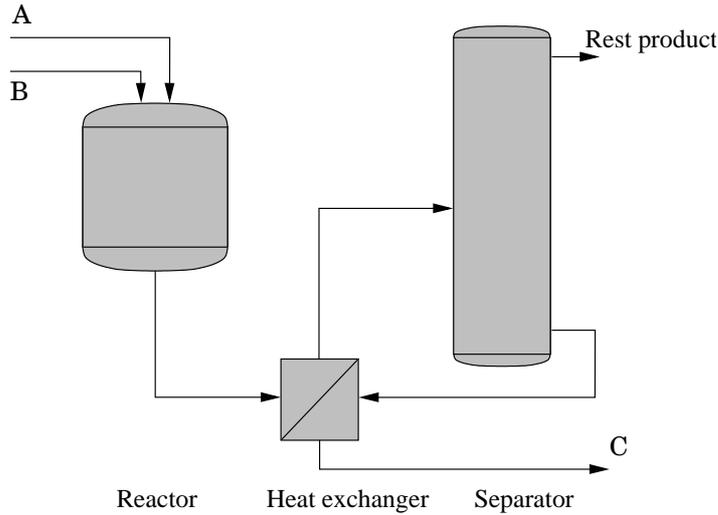
**Figure 1.8** Process flowsheet for a simple plant with a reactor, heat exchanger, and a distillation column.
