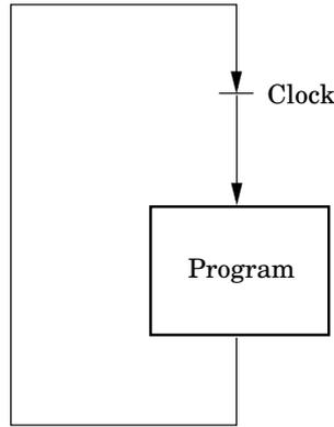
**Figure X.12** A simple operating system.
