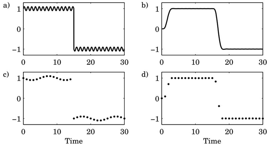
**Figure X.7** Usefulness of a prefilter. a) Signal plus sinusoidal disturbance; b) The signal filtered through a sixth-order Bessel filter; c) Sample and hold of the signal in a); d) Sample and hold of the signal in b).
