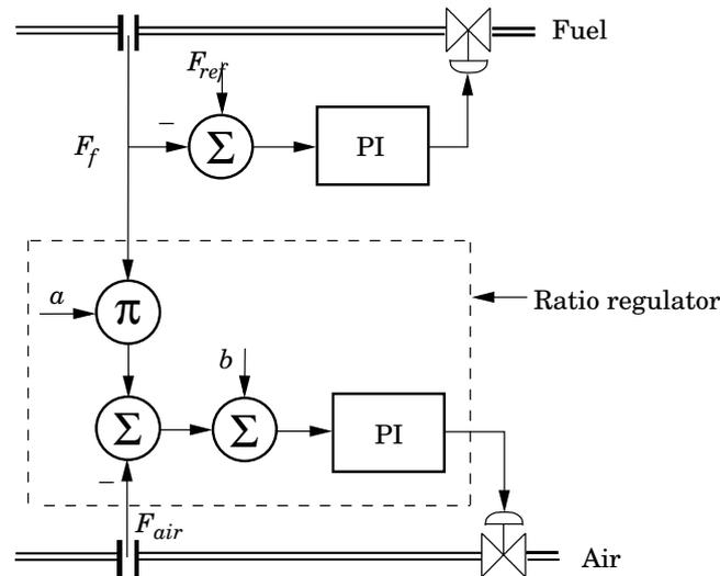
Figure 10.8 Configuration for air/fuel ratio control to a boiler or a furnace.
