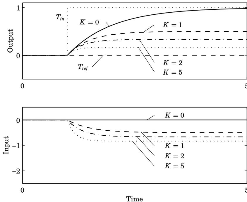
**Figure 6.6** Simulation of the stirred tank under P control with  $K = 0, 1, 2,$  and  $5$ . The desired reference is  $T_{ref} = 0$ , and the disturbance is a unit step at  $t = 0$ . The case  $K = 0$  gives the open loop response.
