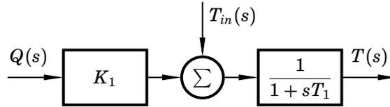
Figure 6.4 Block diagram of the stirred tank process.
