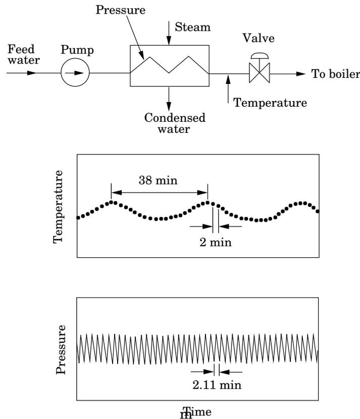
**Figure X.6** Process diagram for a feedwater heating system of a boiler.
