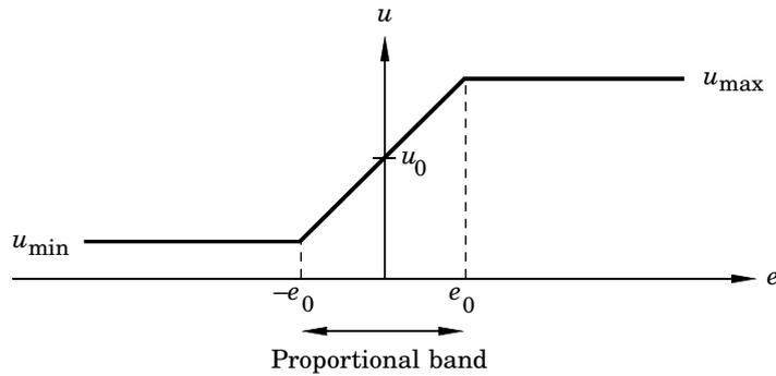
Figure 2.7 The control signal of the P controller.
