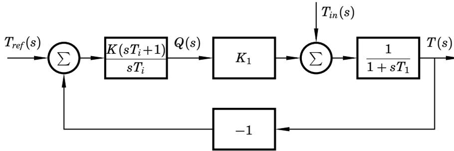
**Figure 6.7** Proportional–integral control of the stirred tank process.
