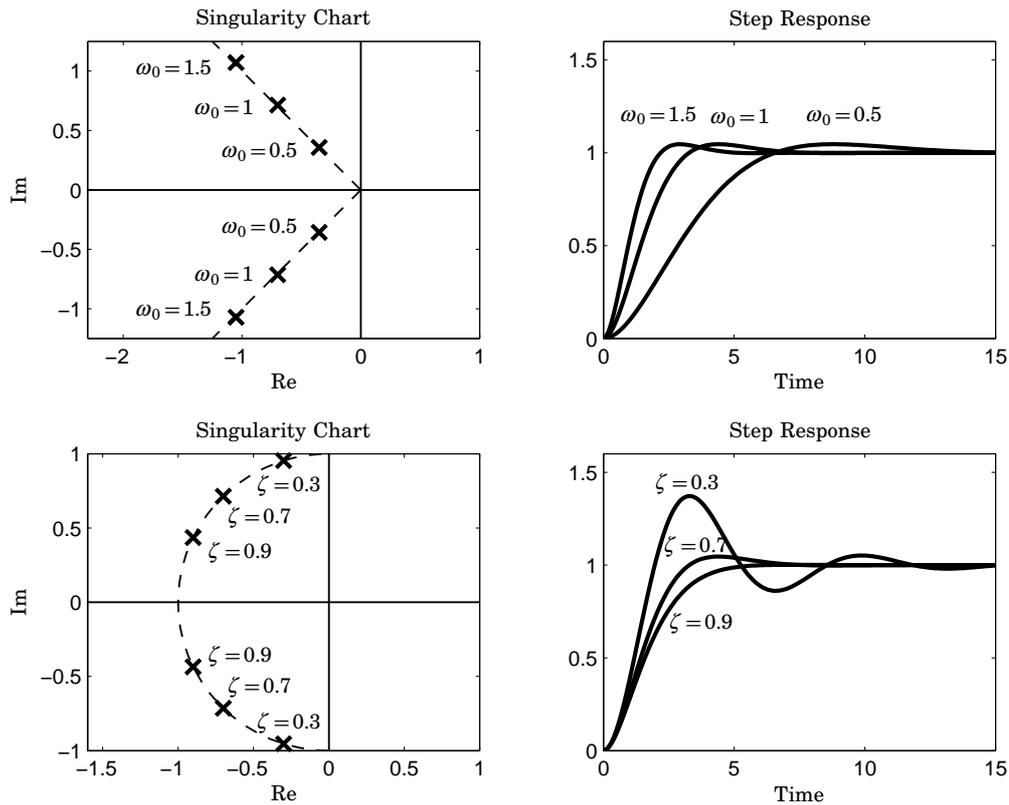
**Figure 5.7** Singularity chart and step response of the process  $G(s) = 1/(s^2 + 2\zeta\omega_0s + \omega_0^2)$ . The two upper plots show the cases  $\zeta = 0.7$  and  $\omega_0 = 0.5, 1, 1.5$ . The two lower plots show the cases  $\omega_0 = 1$  and  $\zeta = 0.3, 0.7, 0.9$ .
