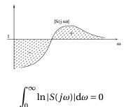
when L has no open RHP zeros and its relative degree  $\geq 2$ .
