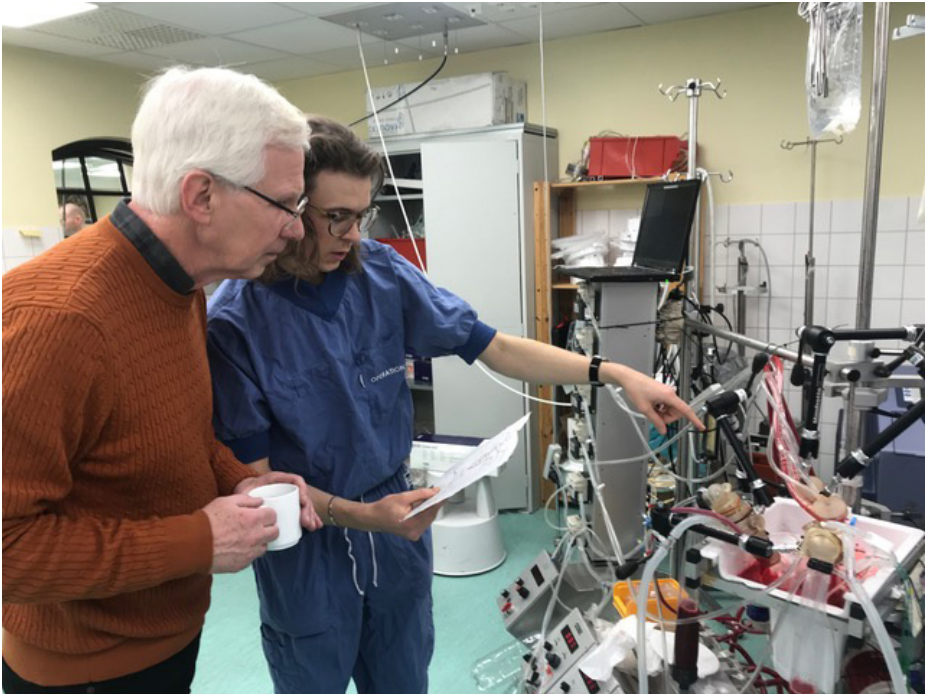
Research setup for ex vivo evaluation and hemodynamic stabilization of heart. The setup relies on soft sensors for state estimation and feedback control for robust performance
