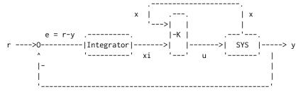
[K,S,E] = lqi(SYS,Q,R,N) calculates the optimal gain matrix K given a state-space model SYS of the plant and weighting matrices Q,R,N. The control law u = -K z = -K [x;xi] minimizes the cost function
