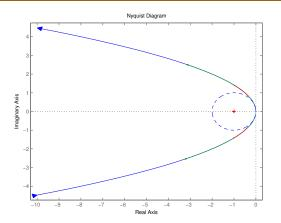
The distance from the loop gain  $L(i\omega I-A)^{-1}B$  to -1 is never smaller than 1. This is always true when  $Q_1>0$ ,  $Q_{12}=0$  and  $Q_2>0$  is scalar. The phase margin is  $\geq 60^\circ$  and the (positive) gain margin is infinite!
