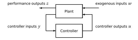
General objective: find a controller that optimizes the closed-loop system  $G_{zw}(s)$ .
