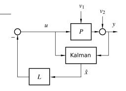
$$\min_{K,L} \mathop{\mathbb{E}}_{v_1,v_2} \left\{ x^T Q_1 x + u^T Q_2 u \right\}$$
