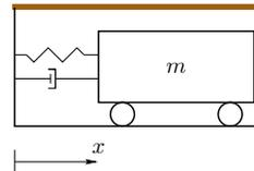
$$m\ddot{x} = - \underbrace{b\dot{x}}_{\text{damping}} - \underbrace{k_0x - k_1x^3}_{\text{spring}}$$
