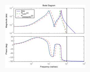
Sample the controller in the same way as the physical plant model is sampled
