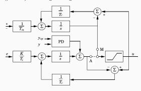
The inactive mode tracks the active mode
