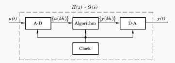
Controller G(s) is designed based on analog techniques
