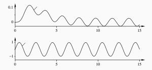
Given a stable system G(s), the input  $u(t)=\sin\omega t$  will, after a transient, give the output
