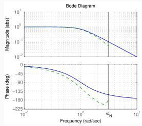
The hold circuit can be approximated by a delay of  $\hbar/2$
