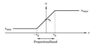
u<sub>0</sub> can be chosen to eliminate stationary error at setpoint
