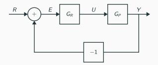
where R, E, U, Y are the Laplace transformations of the reference r(t), control error e(t), control signal u(t), and output y(t), respectively.
