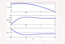
The position on the road, y, moves initially in the intended direction, but due to fork dynamics then in the wrong direction
